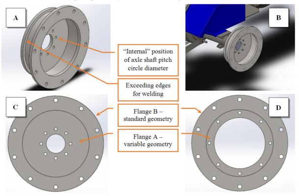
Fig. 6. Version 2 of the adapter: A – 3D drawing with the parts in evidence; B – example of installation on a tractor; C and D – example of two adapters for different rim classes
