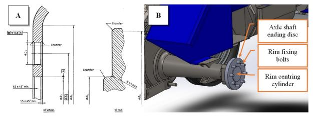
Fig. 3. Wheel-to-hub fixing dimensions from ISO 5711 Standard (A) and example of fastening system on the tractor axle shaft hub (B):  $D_1$  – pitch circle diameter;  $D_2$  – stud hole diameter;  $D_3$  – central bore diameter;  $D_4$  – disc flat bearing diameter;  $D_5$  – centring diameter on the hub;  $D_6$  – diameter of the hub flat bearing)
