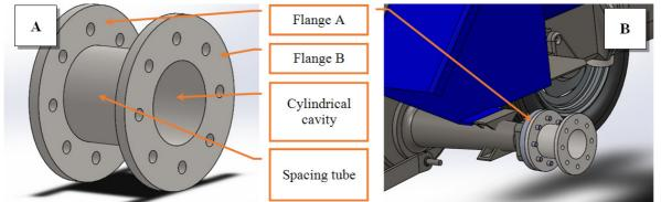
Fig. 5. Version 1 of the adapter: A – 3D drawing with the parts in evidence; B – example of installation on a tractor
