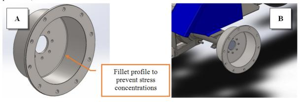
Fig. 7. Version 3 of the adapter: A – 3D drawing; B – example of installation on a tractor
