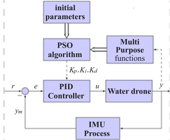
Fig. 11. Block diagram of PSO with the use of PID Controller
