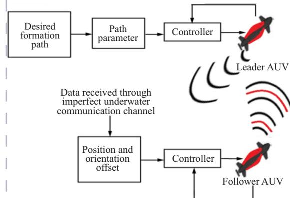
Fig. 4. Signal Control flow for Swarm-communication
