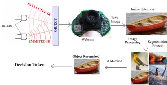
Fig. 2. Intruder detection and recognition scenario
