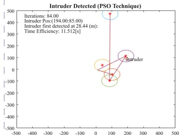
Fig. 18. Surveillance of 5 swarm robots with Intruder detection capability
