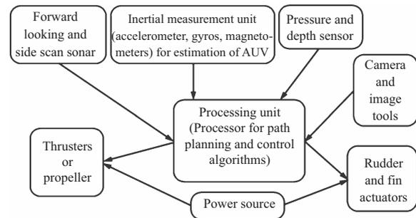
Fig. 1. conceptual diagram of underwater swarm robots
