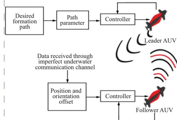
Fig. 4. Signal Control flow for Swarm-communication
