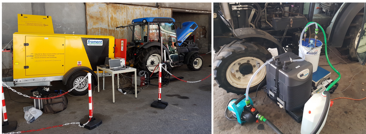
Fig. 2. Complete test-layout for farm tractor at the dyno (left); particular of fuel-consumption meter system placed at the left side of tractor (right)
