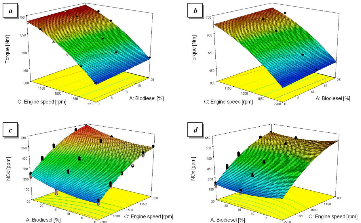
Figure 2 – Surface plot of the engine torque (a and b) and the NO<sub>x</sub> concentration in the exhaust gases (c and d) as a function of the biodiesel percentage and of the engine speed, with the 0 % (a and c) and the 3 % (b and d) of bioethanol in the blend.
