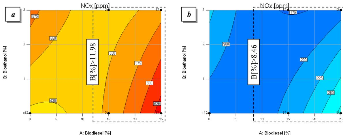
Figure 3 – Contour plots of the NOx concentration as a function of the bioethanol and biodiesel percentages (full ranges of concentration), at 1121 rpm (a) and 2991 rpm (b); the values of NOx are reported as labels directly on the contours.
